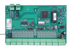
The PRO-2200 Series family of access modules is controlled by and connected to the intelligent control module through a supervised RS-485 bus at 38,400 bps. Hardware interface configuration options are stored in the intelligent control module and may be directly controlled via operator intervention, time schedules or event-based procedures.
