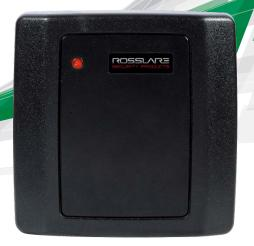
Rosslare's AY-MR12B is a powerful RFID proximity card reader of 125 KHz cards and tags, featuring Wiegand 26-Bit output format and a read range of up to 10 cm (3.9 in.). With a sleek design and a tough UV-resistant and water-resistant casing, the AY-MR12B is equally suited to indoor and outdoor use and is both economical and reliable.
